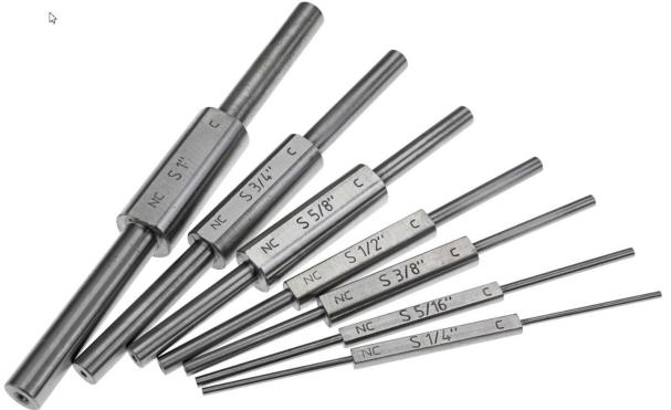
The performance of a hose assembly in terms of its resistance to blow-off and leakage is determined by the level of hose wall compression achieved during the swaging process. Insert bore collapse is used as a method of checking the correct compression level and sealing force.
